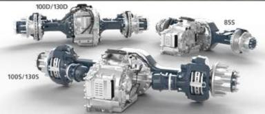
Fully Integrated Electric Axles
